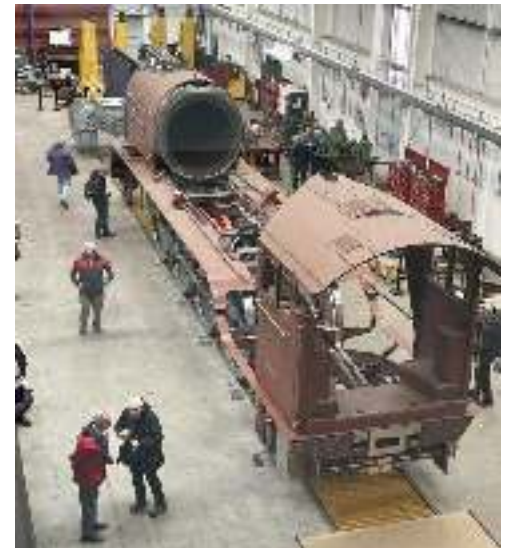
View of the P2 from the overhead gallery - substantially complete, but lacking its boiler!
